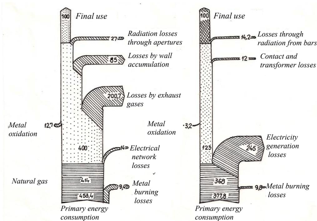
Fig.2.2. Sankey energy diagrams for metal warm up processes:
